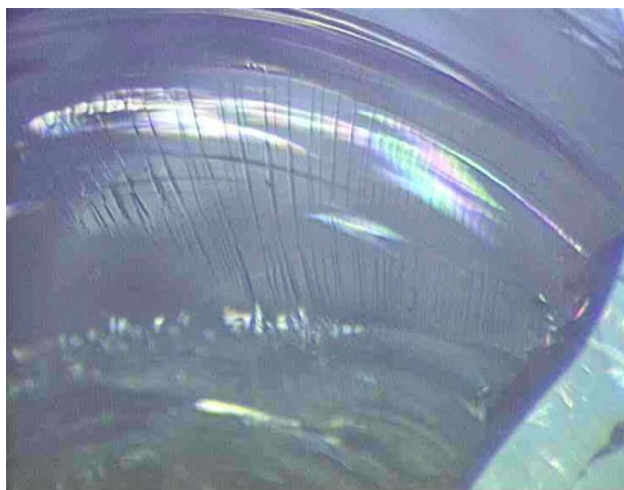
Fig. 7 Formation of fracture lance fronts ( F = 1.839 kN; image width: 3 mm)
